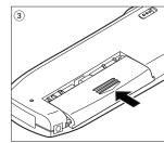
③Make sure that the polarity of each battery is correctly aligned as indicated, then slide the battery cover completely closed.
